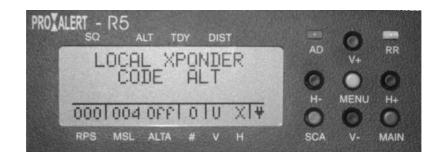
Your local transponder code and altitude, as provided by your aircraft altitude encoder, are displayed if your aircraft is under radar coverage. Any significant discrepancy between your altitude (as reported by your aircraft altimeter set to the standard pressure 29.92" or 1013 Hpa) and the R5 transponder test should trigger servicing your transponder.
