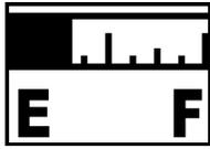
You can also specify 2 to 5 alarm zones for this type of gauge. The alarm zones are fully programmable. You can select attributes such as; number of zones, zone upper and lower limits for each zone, alarm dwell time, alarm self-reset, color, & etc. You can also select the zero and full scale calibration points for a given input signal.
