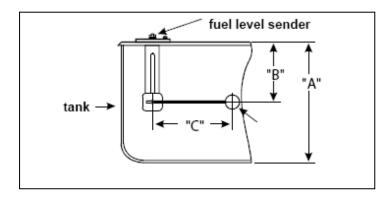
Diagram A Measurements Needed to Make Proper Adjustments
