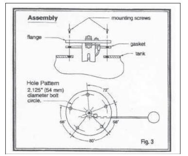
3. Slip the fuel sender assembly into the 2.322"(59mm) hole in the tank, turning assembly until it goes into the tank.
