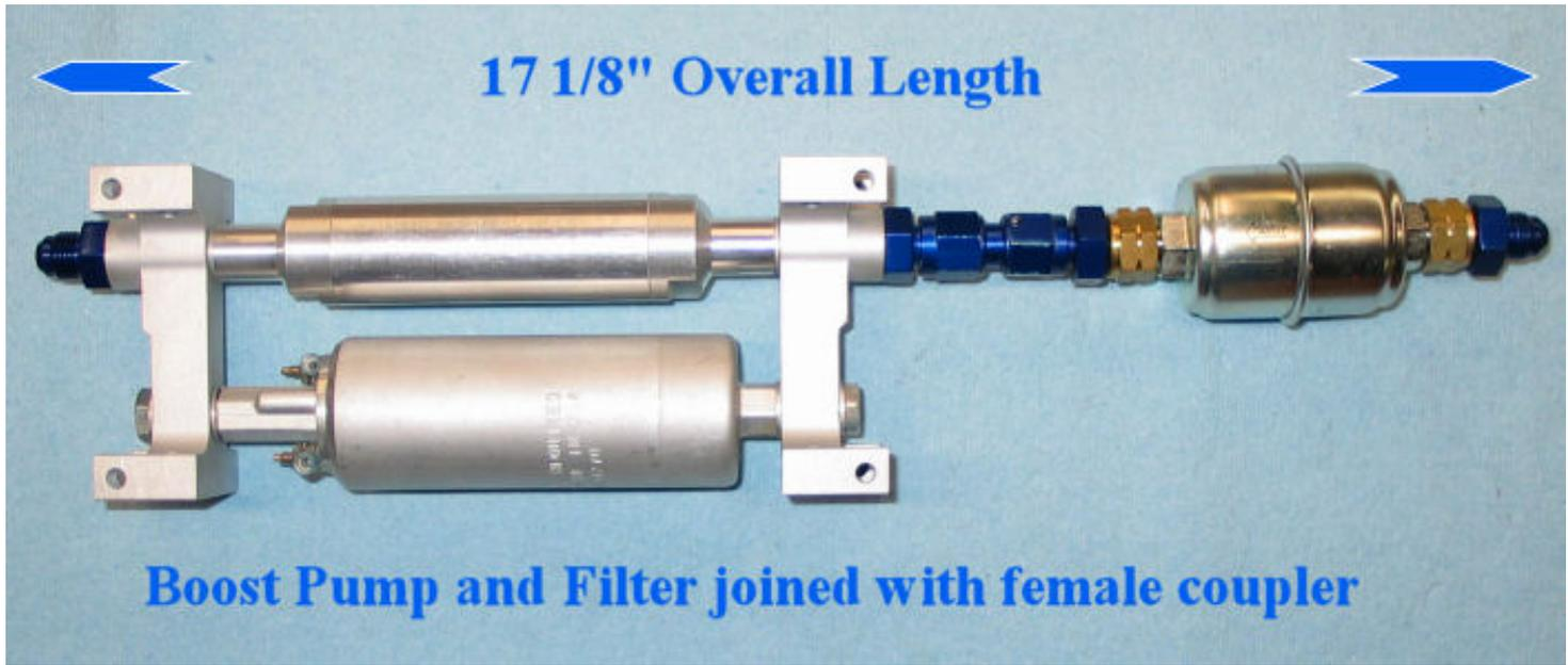
of 17 1/8". In some cases it is desirable to have a shorter installed length of the components. This can easily be accomplished by mounting the fuel filter directly onto the Boost Pump, thereby saving the length of two fittings.
