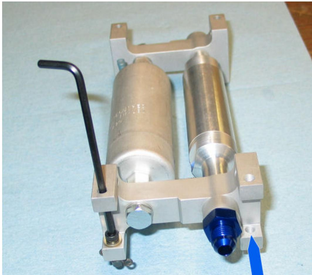
Pump Module. In the photo, the washer on the right has been trimmed a bit on one side to provide clearance with the manifold portion of the Boost Pump. The washer on the left side does not require the trim do to the shape of the manifold.
