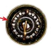
Washer abuts at a 90° shoulder on tapered axle.
