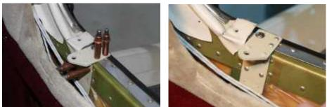
5. Airframe Bracket utilized existing Slide lock screw attachment
