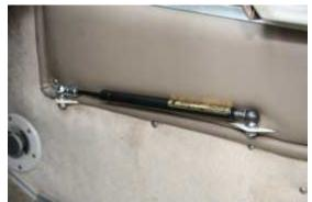
Picture 9. Closed Note door bracket mounted up slightly to avoid contact on the wind lace.
