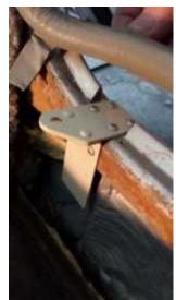
7. Any door sill windlace will need to be trimmed or slit to accommodate going around the installed airframe bracket. Picture 11.
