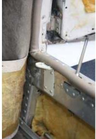
Picture 4. Bracket riveted, wind lace reinstalled between layers
