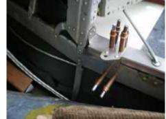
Picture 2. Airframe Bracket Clecoed in place.
