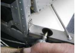
Picture 1. Cutting out sill area (Not Required on All Installations)
