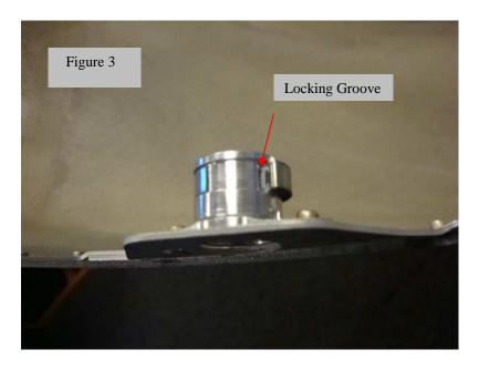
Upon the initial reinstallation of the cowling, engage the SK28S3 studs into the receptacle and screw the studs to the proper set position. Push and turn to unlock studs without disturbing the inserts. Remove the cowling. Turn each insert to align the "slot" with the rivets. With the pick tool, snap the clips back into the locking groove and check that the insert is locked (the slot will be a few degrees past being aligned with the rivets).
