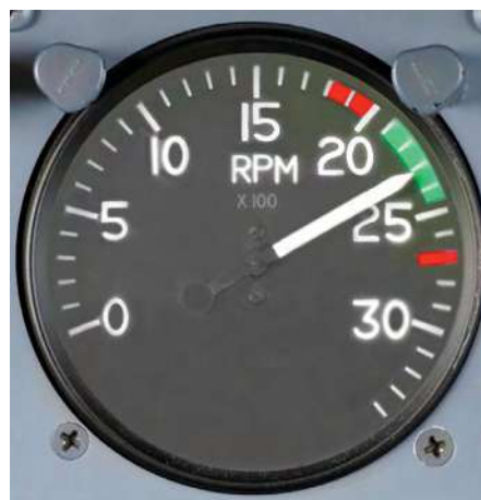
Figure 1-17. Red arc from 1 800 to 2 000 rpm.
