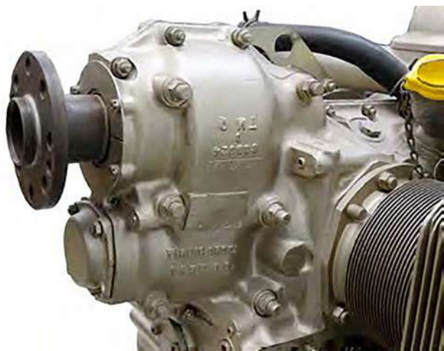
Figure 3-31. Spur-Type propeller gear reduction system.
