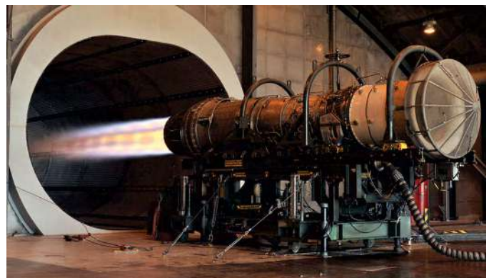
Figure 2-1. Gross thrust from a static turbojet engine.
