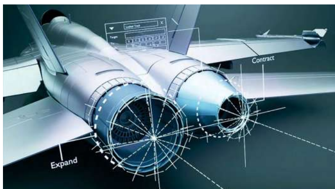
Figure 2-2. Variable exhaust ducts on military aircraft create convergent or divergent conditions.
