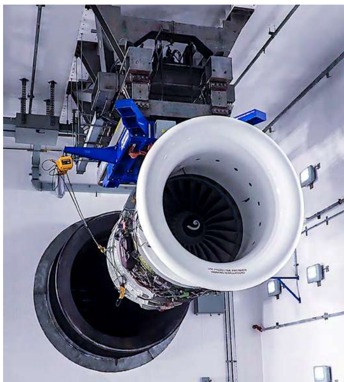
Figure 3-15. Bellmouth inlet mounted on test cell engine.
