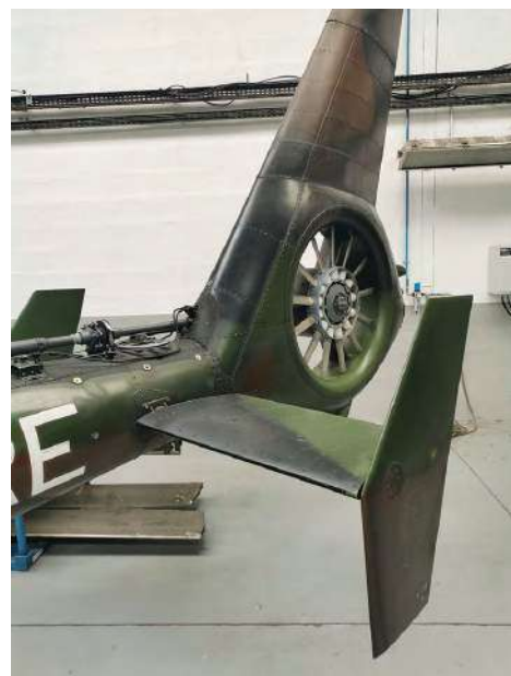
Figure 2-27. Fenestron on a Eurocopter Model SA341 Gazelle.
