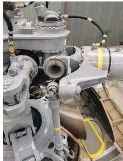
Figure 2-33. Fully Articulated Main Rotor System.
