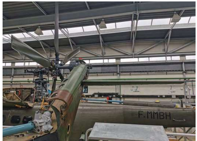
Figure 2-26. Aerospatiale Helicopter Tail Rotor.
