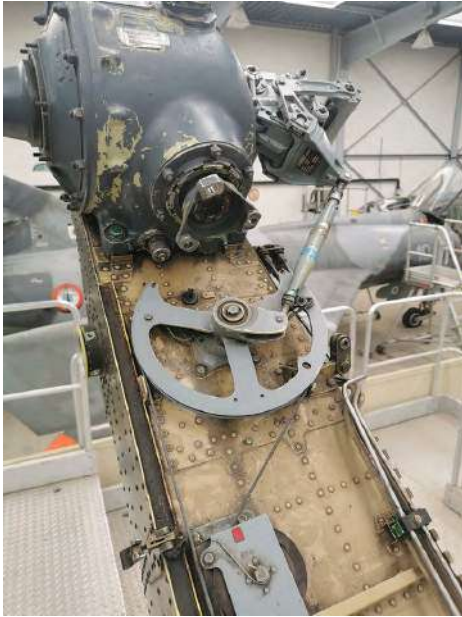
Figure 2-23. Cables-rear sector-rod and tail servo-control.
