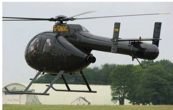
Figure 2-29. MD-520 helicopter with no tail rotor.
