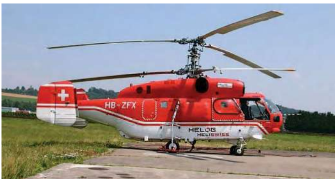
Figure 2-25. Helicopter with coaxial counter-rotating main rotors.
