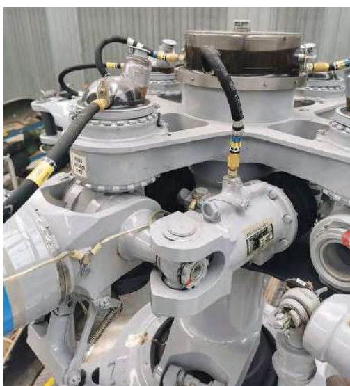
Figure 2-35. Drag hydraulic damper on SA330 puma.
