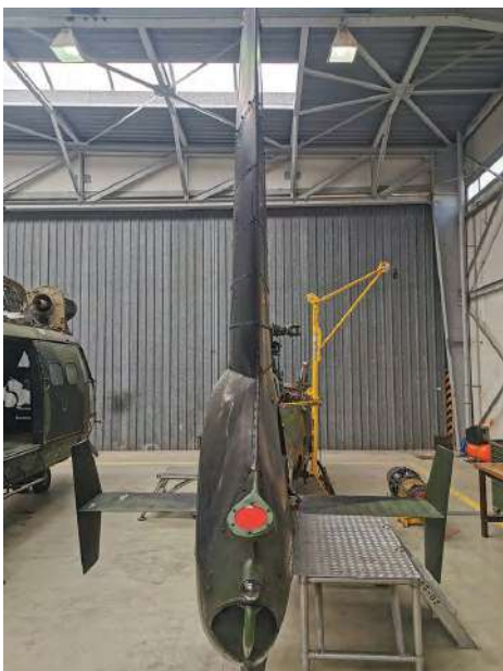
Figure 2-28. Fenestron dissymmetric vertical fin.
