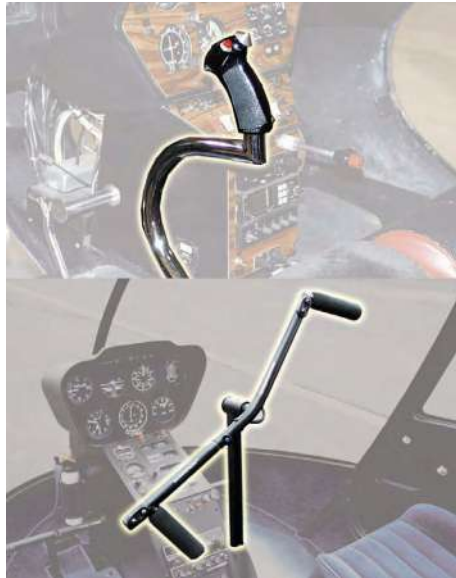
Figure 2-2. Location of cyclic pitch control.
