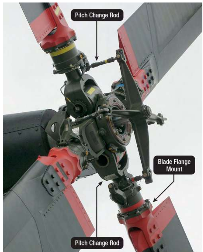
Figure 2-11. Tail rotor description.
