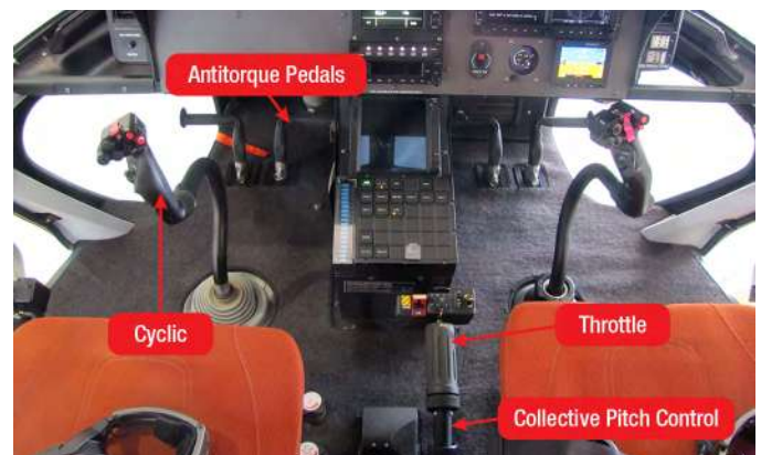
Figure 2-1. Helicopter controls on the flight deck.
