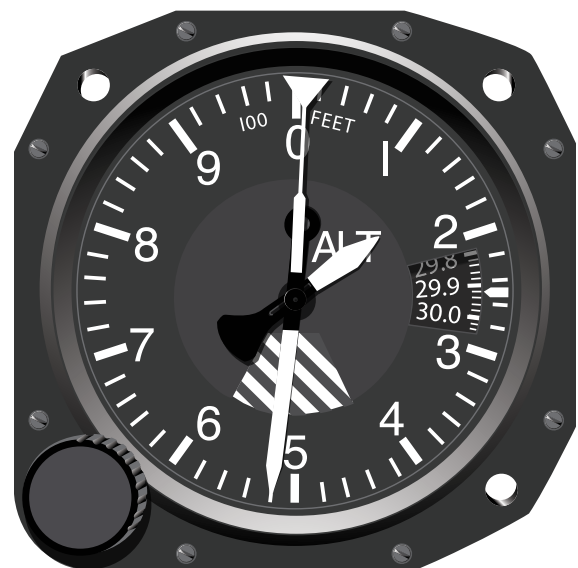
Figure 1-3. An airplane's altimeter is an aneroid barometer.
