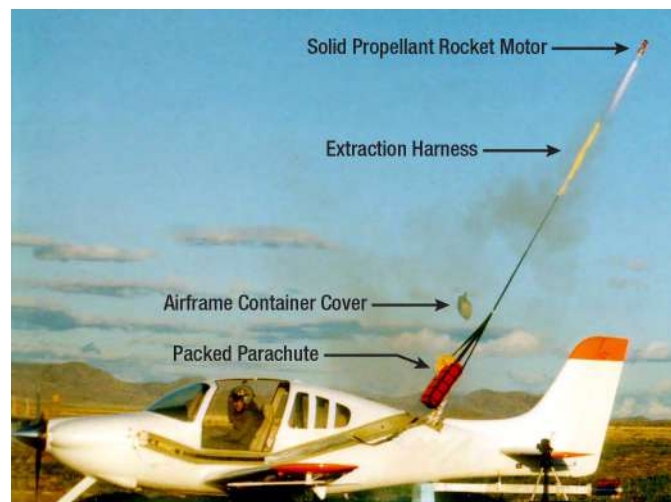
Figure 1-9. The firing sequence of a rocket propelled parachute system.
