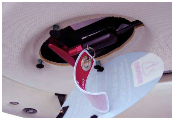
Figure 1-8. An actuation handle with its remove-before-flight safety pin in place.
