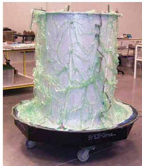
Figure 3-31. Bagging of complex part.
