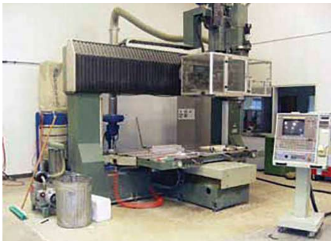
Figure 3-28. Five-axis CNC equipment for tool and mold making.
