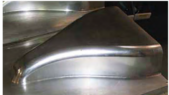
Figure 3-29. A mold of an inlet duct.
