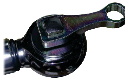
Figure 3-16. A typical torque wrench extension in the straight position.
